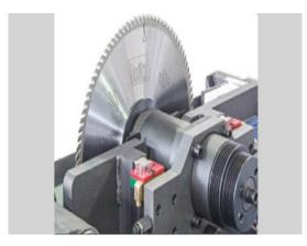
•Linear guide structure cutting system, saw shaft with second dynamic balance treatmenr, with German Leiz saw blade
