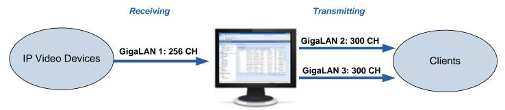
GV-Recording Server + 3 Network Cards assigned on different networks
